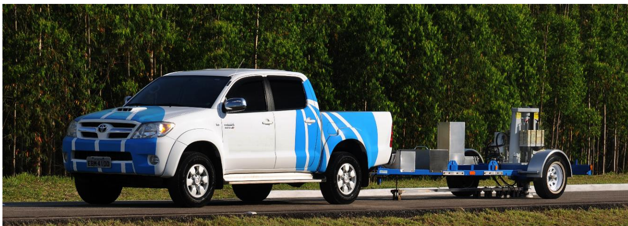
Figura 2 – Vista do Falling Weight Deflectometer Dynatest 8000.
